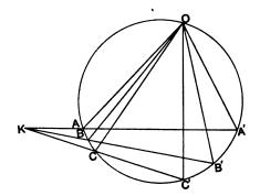
Let any circle be drawn passing through O, cutting the rays of the pencil in the points A, A', B, B', C, C'. Then by § 85, AA', BB', CC' will meet in the same point K.
